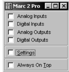
By enabling the checkboxes “*Analog Inputs*”, “*Digital Inputs*”, “*Analog Outputs*”, “*Digital Outputs*” and “*Settings*” further windows are opened, in which you can read and change the appropriate settings. By enabling the checkbox “*Always On Top*” you can always see the opened windows on top of all other application windows.
