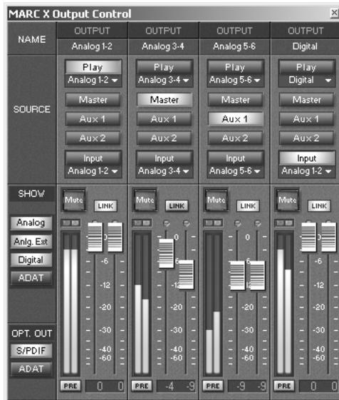
All output settings are performed using the "OUTPUT CONTROL" window. It contains a channel each for all available physical outputs. Within the "OUTPUT CONTROL" window all input signals, playback signal and sum signals can be assigned absolutely flexibly to the available outputs.
