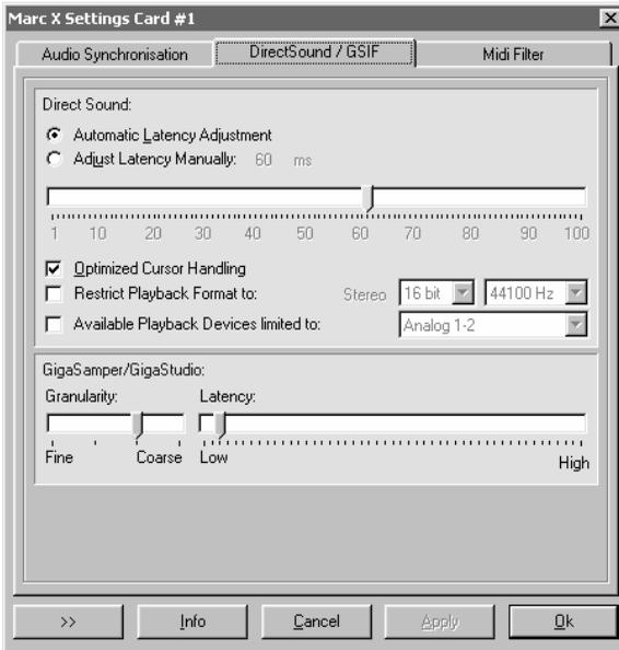
Here you can determine the settings for application programs which use DirectSound or the TASCAM GigaSampler Interface (GSIF) in Windows™ 95/98/ME.
