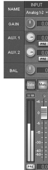
The **GAIN** controllers of the analog inputs influence the level of the source signal.
