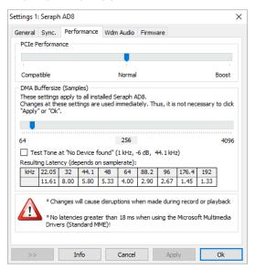
**PCIe Performance** For best results, we recommend the "compatible" option, if the PCIe slot used is connected with the CPU directly. (e.g. 16x slots or small mainboards with just one or two PCIe slots) We recommend the "boost" option for all other, standard cases, where the PCIe slot is connected with a PCIe host controller.
