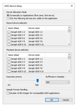
In the field of professional music production on the PC, the ASIO interface has established itself as a standard. The ASIO device setup offers important setup features for using the SERAPH AD8 with an ASIO interface. It is opened from within the audio application that supports the ASIO standard. Mostly there is a button called 'control panel' or 'setup' near the selection field for the ASIO driver. Clicking it will open the ASIO device setup.
