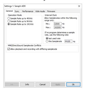
**Operation Mode** The SERAPH AD8 may be operated in 3 different operation modes, chosen here. In 192 kHz mode, the number of mixing sums is reduced to 4. Consequently, there are 2 aux-sums ('Aux 1' and 'Aux 2') besides the main mixing sum.
