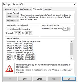
This settings window allows for changes that apply only to the WDM driver part of the SERAPH AD8. ASIO and other driver interfaces remain unaffected.
