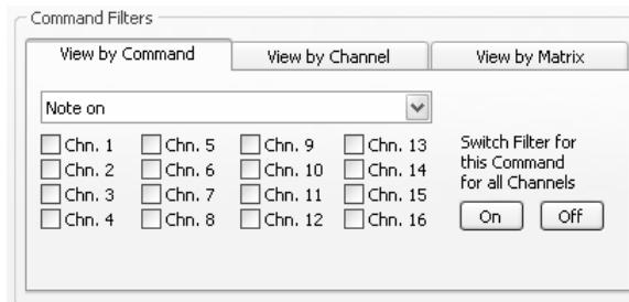
On “View by Command”, “Command Filters” shows the MIDI commands, which can now be filtered for each single channel. By clicking “On” or “Off”, the chosen MIDI command is filtered or passed through on all channels.
