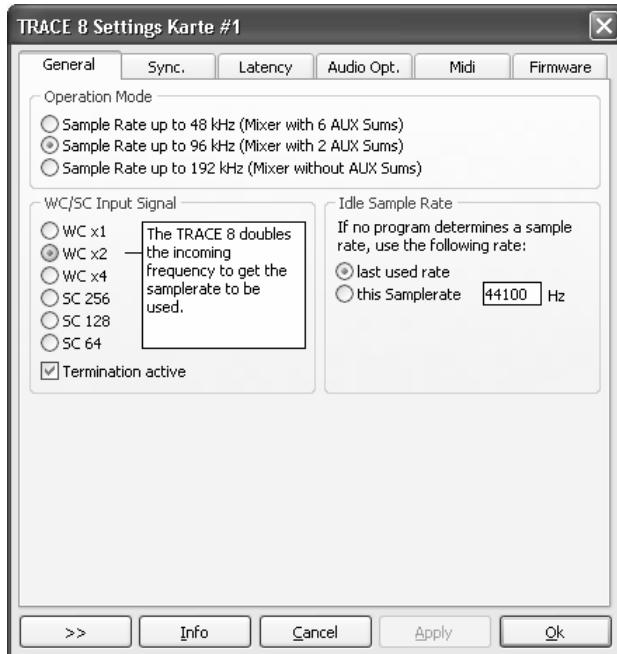
The following chapter is all about the system settings of the TRACE 8. You open the corresponding window via the TRACE 8 symbol on the taskbar. Should questions remain, we recommend taking a look at the “hands on”-part of this manual. Especially the section “The TRACE 8 in connection with digital devices” contains simple examples for right handling of the clock settings.
