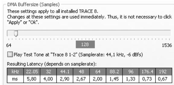
▷ *The DMA buffer size is always simultaneously changing the latency for the GSIF interface.*
