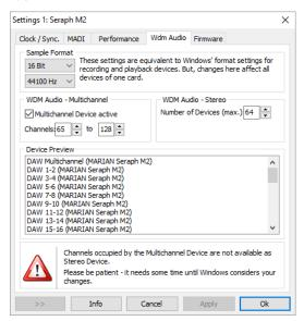
This settings window allows for changes that apply only to the WDM driver part of the SERAPH M2. ASIO and other driver interfaces remain unaffected.
