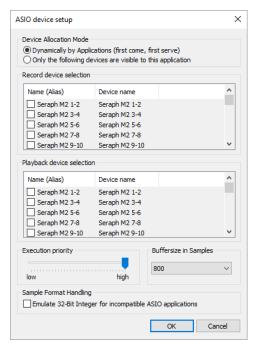
In the field of professional music production on the PC, the ASIO interface has established itself as a standard. The ASIO device setup offers important setup features for using the SERAPH M2 with an ASIO interface. It is opened from within the audio application that supports the ASIO standard. Mostly there is a button called 'control panel' or 'setup' near the selection field for the ASIO driver. Clicking it will open the ASIO device setup.
