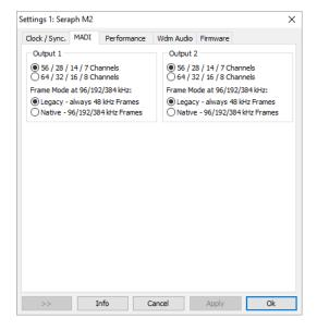
Output 1 / Output 2 A MADI channel may be operated in 2 modes. Changing between 56 channel- and 64 channel mode may be done for each MADI output separately in this section.
