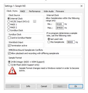
**Internal Clock** In this section the operation limits of the SERAPH M2 may be defined using the 'min' and 'max' entry fields.
