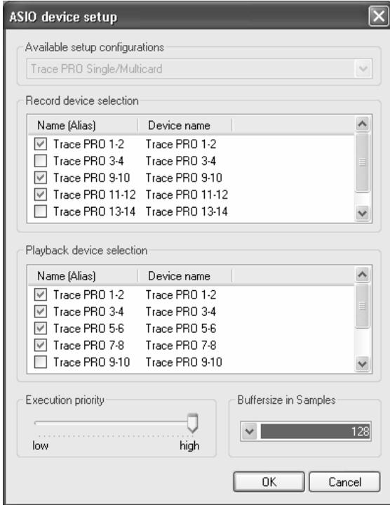
Due to small latency time, the ASIO interface has become a standard in professional music production. The ASIO device setup offers important settings for the TRACE PRO using the ASIO interface. It is opened from within the audio application, which supports the ASIO standard. Most times there is a button called “control panel” next to the field where the ASIO driver is selected – a click on it opens the ASIO device setup.
