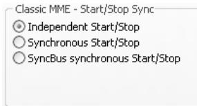
The start/stop synchronization can be turned on or off for all audio devices. If this option is active, the audio data transfer of all audio devices is started and stopped simultaneously.
