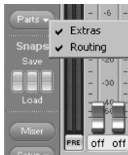
You may save certain visual configurations along with the current Output Control settings in a “snapshot”. For this, click on one of the three buttons beneath “snaps” on the row “save”. If you wish to recall a snapshot, click on the
