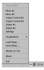
$\triangleright$ If several TRACE PRO AEhave heen installed, the entries for Mixer and Output Control will appear accordingly with the extension  $,, #2^{\circ},$ .. #3 '' and so on. The the sound settings of systems are managed via one window.
