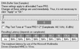
▷ The DMA buffer size is always simultaneously changing the latency for the GSIF interface.
